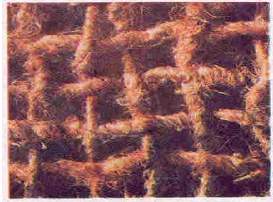
Close-up view of conventional jute geotextile (geojute)
